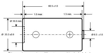
Dimensions are in millimeters and include label.
